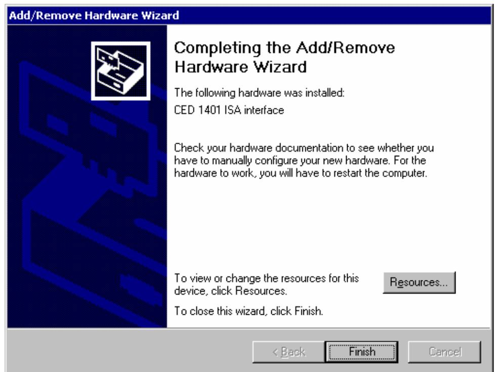
**The I/O base address** The installer sets a default I/O base address of 300. This matches the default address set by links on the interface card (see page 25 for details.) If you are using this default address, simply press *Finish* to complete the installation. If your card's address has been altered, e.g. to avoid clashes, the software I/O address must be set to the correct range before installation. Changes to interrupt and DMA channel are dealt with automatically.
