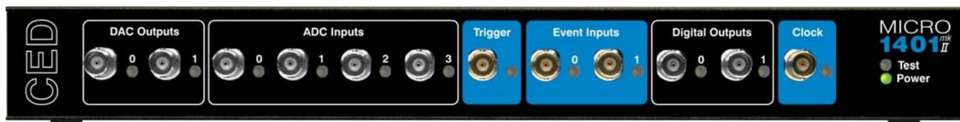
**Clocks** The Micro1401 has five clocks, used for timing and counting external pulses (clocks 0 and 1), generating general purpose timing pulses (clock 2), controlling waveform output (clocks 3 and 4) and controlling the waveform input sampling rate (clock 4). These clocks are managed automatically by the application software.
