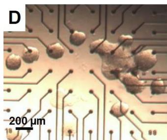
*Microscopic view of islets cultivated on the electrode field of a MEA for long-term recordings.*
