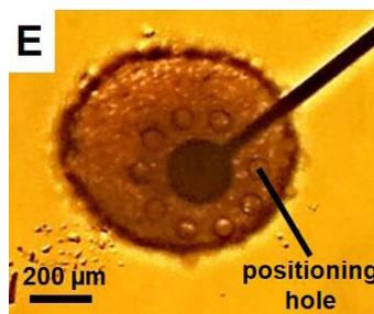
*View of a Beta-Screen electrode covered with an intact murine islet positioned via negative pressure through the positioning holes.*
