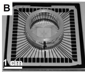
*Islet of Langerhans placed on top of a MEA electrode during an acute measurement.*
